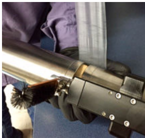
Figure 1 Parafilm® to be wound around optical area
